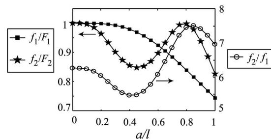
FIG. 4. The resonance frequencies ratios change with the position of the attached mass. It can be seen that the shift on  $f_2$  is more significant than  $f_1$  when the mass is close to the clamped end of the beam while the frequency shift on  $f_1$  is more significant than  $f_2$  when the mass is close to the free end.
