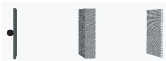
Figure 3: MPM simulation model of the filling Whipple shield structure
