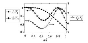
FIG. 4. The resonance frequencies ratios change with the position of the attached mass. It can be seen that the shift on  $f_2$  is more significant than  $f_1$  when the mass is close to the clamped end of the beam while the frequency shift on  $f_1$  is more significant than  $f_2$  when the mass is close to the free end.
