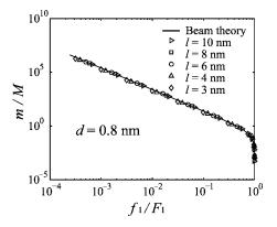
FIG. 2. The changes of the frequency ratio corresponding to the mass ratios obtained by the membrane-spring model for SWNTs samples, and compared with the result of LBT. The data of SWNTs with length larger than 4 nm agree well with the one of LBT.
