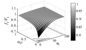
FIG. 3. The variation of the frequency ratio with the position ratio  $a/\ell$  and the stiffness ratio  $\eta = k \ell / EI$  of the volume defect. It indicates that when the position of the volume defect is closer to the clamped end, the influence is more significant.
