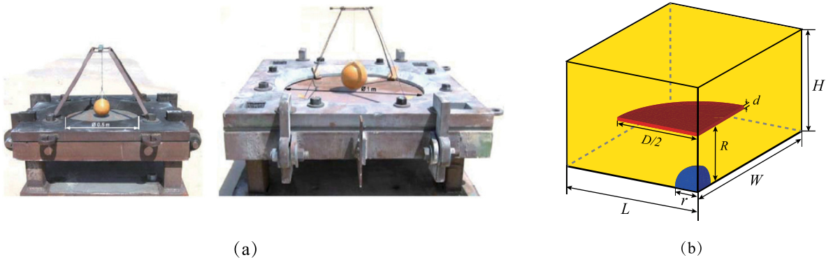
Fig. 13. (a) The experiment devices [80] (b) Blast-plate interaction. (For interpretation of the references to color in this figure legend, the reader is referred to the web version of this article.)
