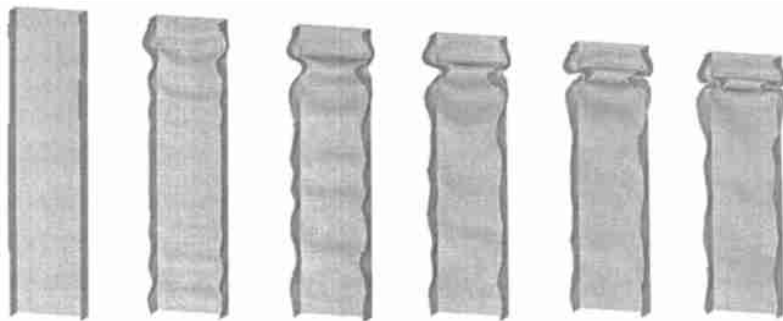
图4 薄壁箱形梁在冲击载荷作用下的变形过程 [8] Fig.4 Large deformation of thin shell structures
